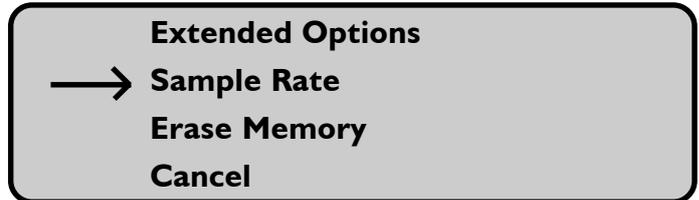
Scroll arrow to sample rate required and press the **ENTER** button. The screen will now return to the Main Menu
