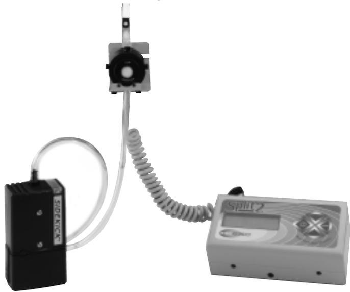
To use in the pumped mode the sensing head must be configured with the appropriate inlet e.g Inhalable, Thoracic or Respirable and with a pre weighed filter in place. The sensor must be mounted on the back plate pointing forward. See the pictures below and on page 13.
