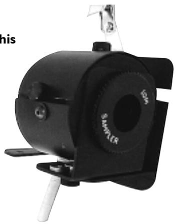
For use in the pumped mode an external sample pump **MUST** be attached as shown. We recommend the SKC **Sidekick** (part # 224-50 or 224-52TX) as your **PREFERRED SAMPLE PUMP**. The pump **must** be set at a flow rate of 2.0 litres/minute
