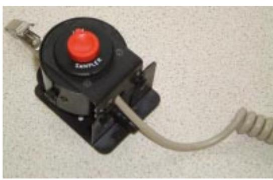
PLEASE NOTE: To configure the sensing head for different dust fraction the IOM inlet with suitable foam is used as shown below. A preweighed filter must also be fitted.
