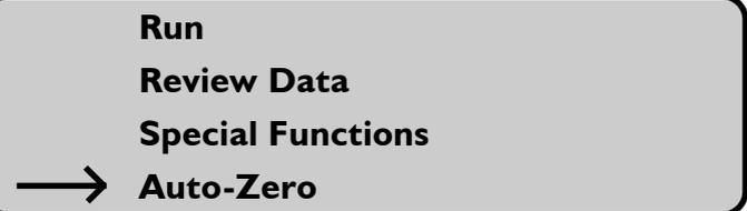
A screen will briefly appear suggesting that the optics are cleaned. To clean the optics, remove the cover of the sensing head. Wipe with a lint free cloth or clean with Isopropyl alcohol. Do not spill IPA over the sensor head as this may cause damage
