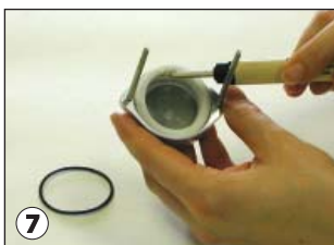
Remove compression ring from outlet plate. See Figure 2.
