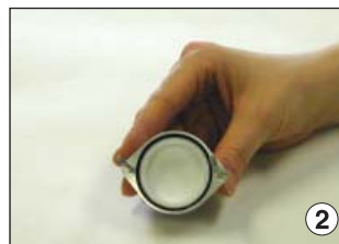
Insert 37-mm after-filter in outlet plate. Replace compression ring and O-ring.
