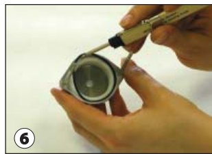
Remove O-ring from outlet plate. See Figure 2.
