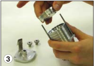
Lift off together accelerator plate A and collector plate.
