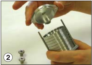
Remove inlet plate.
