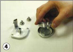
Lift accelerator plate A off collector plate.
