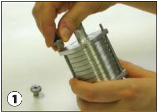
Remove thumb nuts.
