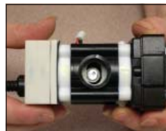
Incorrect: Eccentric off-center and binding yoke.
