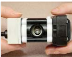
Correct: Eccentric centered in yoke.
