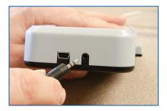
b. Insert other connector end of cable into CalChek port on back of charging cradle (e-Cradle shown).
