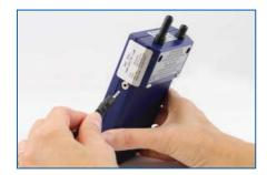
a. Install one connector end of cable into CalChek interface socket on flowmeter.
