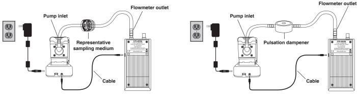
Figure 3. CalChek Single Calibration Train
