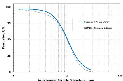
Collection efficiency of the 2 L/min thoracic PPI Sampler compared to the ISO thoracic convention
