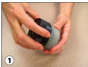
Unscrew the inlet from the exhaust.
