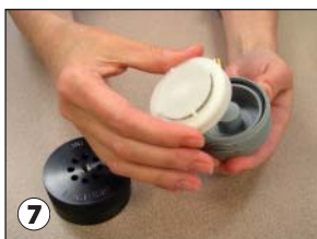
Reinsert the cassette into the impactor.
