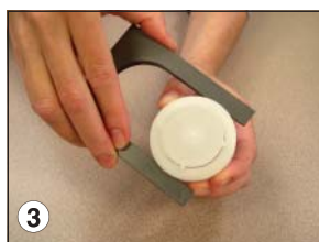
3a. Use the filter cassette opener to open the filter cassette.
