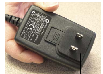
Interchangeable wall plugs slide into power supply.
