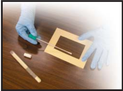
Surface Swab Kit contains 10 sterile swabs in transport tubes and 10 plastic templates (5 x 10 cm)
