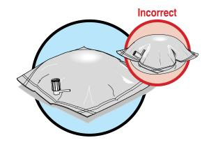
Secure polypropylene valve when opening/closing by holding side stem while turning entire upper portion of fitting one revolution.
