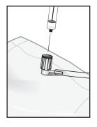
5. To withdraw samples using a needle and syringe, carefully insert the needle into the syringe port in the center of the brown or white septum cap and pierce the septum.
