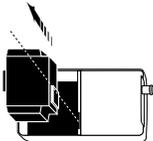
5. Completely charge the new battery pack **detached** from the pump. This initial slow charge will provide optimum battery performance.
