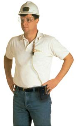
Clip holder to worker and pump to belt
