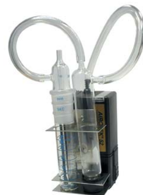
Impinger holder on pump with impinger and trap
