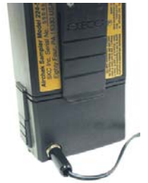
Charger and battery connected
