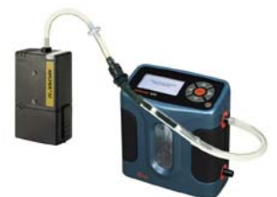
Calibration train with tube in low flow holder
