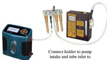
Connect holder to pump intake and tube inlet to flowmeter.
