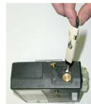
For low flow, turn valve screw counterclockwise.
