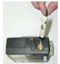
For high flow, turn valve screw clockwise.
