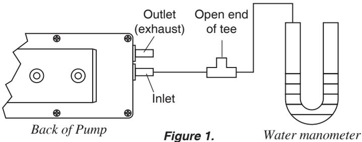
2. On the open end of the tee, draw vacuum by mouth until 4 to 5 inches of water vacuum register on the manometer.
