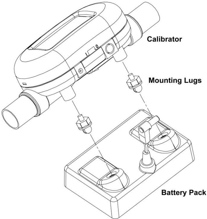
Figure 2-1 Calibrator Assembly
