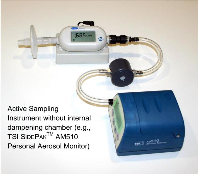
**Figure 2-3 Typical Dampening Module Set Up**
