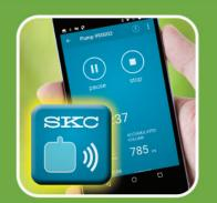
Bluetooth<sup>®</sup> connection for pump operation and monitoring from phones and tablets.
