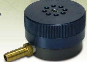
The patented\* SKC IMPACT single-stage inertial impactor is designed for efficient collection of PM10, PM2.5, or PM Coarse (10-2.5) in ambient air. Operated at 10 L/min constant flow, larger particles are captured on a disposable pre-oiled impaction disc while smaller particles collect on a 47-mm filter. The filter and impaction disc are housed in a removable filter cassette. The IMPACT's higher flow rate provides increased sensitivity for low levels of PM.
