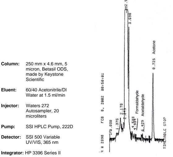
Figure 7. Sample chromatogram - blank DNPH-treated filter in acetonitrile
