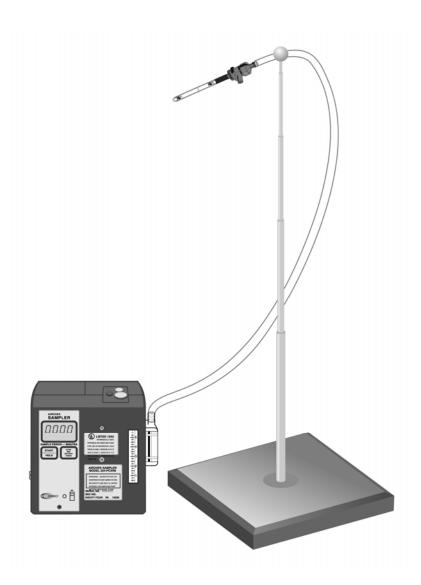
Figure 2. Portable area sampling system for solid adsorbent traps
