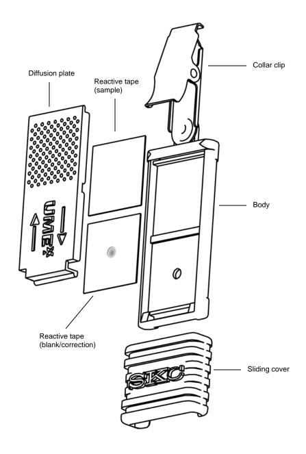
Figure 6. UME<sup>x</sup> 100 Passive Sampler (exploded view)
