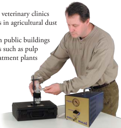
BioSampler set up with BioLite pump
