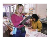
Used for real-time monitoring or concurrent gravimetric sampling, SPLIT2 is comfortable to wear and does not interfere with daily activity. When configured with a sample pump, the SPLIT2 with built-in belt clip can be placed on one side of a worker's belt and the pump on the other side for maximum comfort. The sensor is mounted near the breathing zone for accurate breathing zone measurement. Handheld wand and tripod accessories are available for area monitoring.
