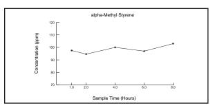
The mean sampling rate was 12.6 ml/min  $(3.65 \mu g/ppm/hr)$  and was calculated as a weighted average of the 1, 2, 4, 6, & 8-hour exposure periods based on a calibrated mean concentration of 99 ppm.
